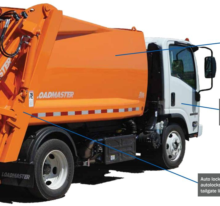
Strong, smooth, curved 10 gauge high tensile body sides. Designed to look good on any chassis. The smooth sides provide a good surface for decals, signs and other advertising. 10 ga high tensile body sides, 10 ga high tensile body roof, 3/16" body floor.
